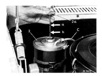
2 Fluid reservoir2a Cover and dipsticka Max. markingb Min. marking
