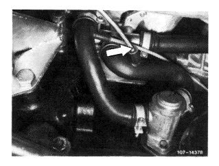
Starting September 1981, the throttle valve housing is provided with 2 connections.
