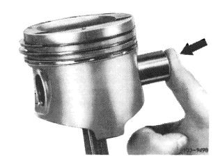
6 Insert piston pin circlips in grooves.
