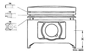
Piston low compression and USA version dimension H = 32 mm
