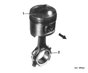
5 Press in piston pin coated with engine oil by hand.
