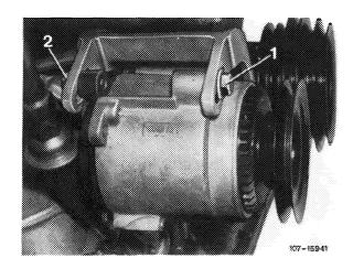
3 Remove V-belt and contoured hose, remove air pump.
