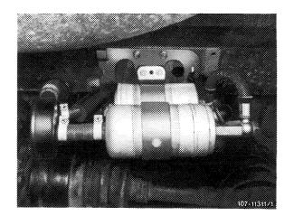
8 Clean fuel pump and fuel filter externally and mount with additional plastic sleeve (slip up to bead of pump).
