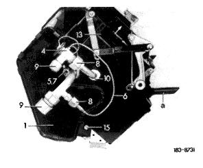
5 Remove sealing strip (10) (NO DRIP TAPE) from expansion valve.
