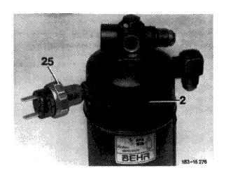
Pressure switch with conical seal
