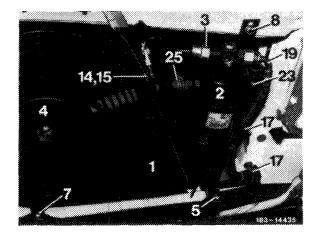
5 To check refrigerant level, pull the two electric plugs from pressure switch and connect to each other (short-circuit). Run air conditioning system for approx. 2-3 minutes, then check immediately after engaging the electromagnetic clutch whether the refrigerant is flowing past receiver dehydrator free of bubbles.
