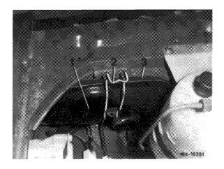
2 Pull coupler (2) from bulb. Unscrew lamp socket (5) from bayonet lock and remove bulb for main headlamp or parking lamp.
