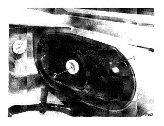
On vehicles with light range regulation, unhook spring clip (2) and remove cover.
