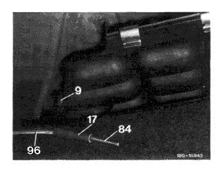
36 Pull suction line (96) out of distributor (22) in engine compartment. Connect tester (refer to arrow) and evacuate.
