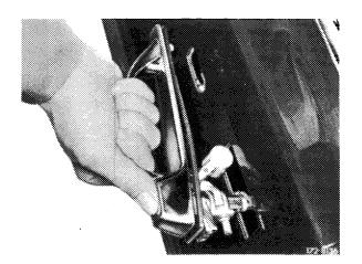
6 Introduce torsion bar (2) into torsion nut (3).
