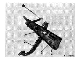
4 Install new rubber stop (3) on bearing tube (4). Install bearing tube with rubber stop in carrier and fasten with a  $8 \times 35$  hexagon head bolt, lock washer and hexagon nut.
