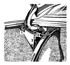
If the electric drive fails, the sliding roof can also be moved by hand. For this purpose a manual drive (1) is provided on the drive motor (LH side of trunk). The manual drive can be rotated by means of adapter (3) retained
