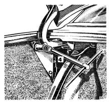
in bracket (2) plus spark plug wrench (4) to move the sliding roof in the desired direction.
