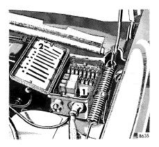
Fuses must not be repaired or bridged.
