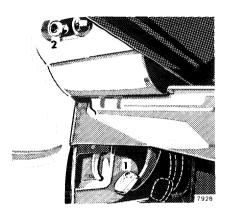
Depress parking brake pedal (1). When the steering lock key is in position "2", the brake warning light in the instrument cluster comes on.
