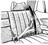
Fastening of rear center belt (without inertia reel):
