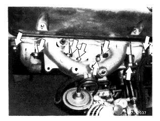
• Retighten bolts of exhaust flanged connections.
