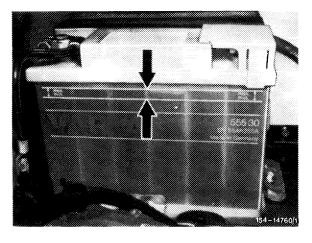
• Check fluid level on batteries where fluid level can be seen.
