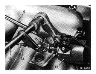
• Connect speedometer to ignition system, Connect inspection lamp to solenoid (12), Run engine at idling speed, Switch-on air conditioner and turn power steering to full lock.
