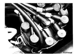
For adjustment, slightly loosen ignition distributor attachment (arrow) and adjust firing point by turning ignition distributor.
