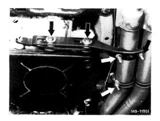
• Detach side support at transmission suspension.
