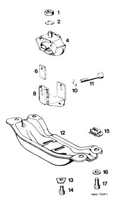
Rear engine mount with engine stop
