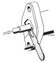
• If the notches are visible, the wear limit of the driven plate has been reached. Exchange driven plate.
