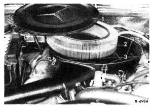
• Blow out element with compressed air from inside max. 5 bar (atü).
