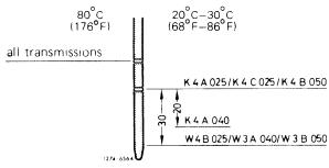
• At a transmission oil temperature of 20 – 30°C (68-86°F) and correct oil level, and depending on type of transmission, the indication should be either at min, mark or correspondingly lower.
