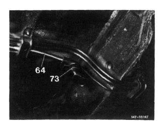
A diaphragm in vent sleeve increases pressure in fuel tank by approx. 10 mbar.
