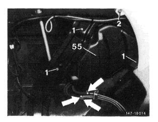
The expansion tank is provided with two connecting lines (arrows) entering the fuel tank and a vent line (64).
