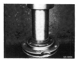
5 Coat O-ring on counterring with brake cylinder paste and push with chamfered side (arrow) into thoroughly cleaned impeller.
