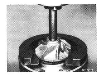
2 Apply light hammer blows at several points between bearing housing and sliding ring seal to cancel the preload and force sliding ring seal out.
