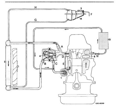
Circuit at coolant temperatures above approx. 94 °C
