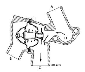
At coolant temperatures of approx. 80 °C up to approx. 94 °C the main valve as well as the bypass valve are more or less open depending on engine load. The coolant flows via radiator (A) and bypass line (C) to coolant pump.
