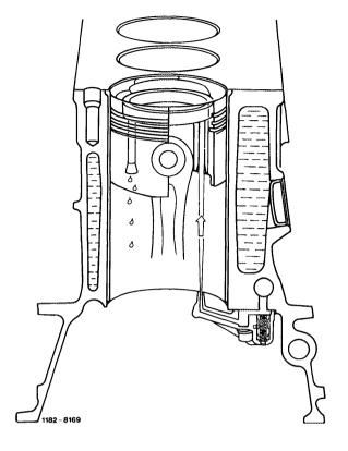
Starting at an engine oil pressure of 1.0-1.5 bar gage pressure, the valve located in oil spray nozzle opens.
