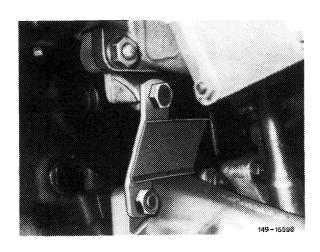
5 Unscrew fastening nuts for intake manifold and exhaust manifold, remove intake manifold and exhaust manifold together with exhaust gas turbocharger.
