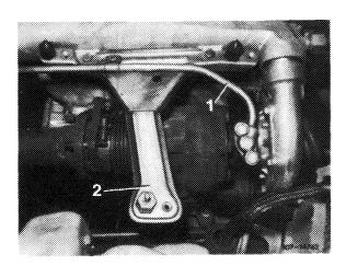
4 Unscrew supporting bracket for exhaust manifold on engine carrier.
