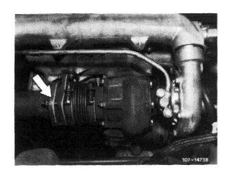
3 Unscrew engine oil feed line (1) on exhaust gas turbocharger and fastening clamp.
