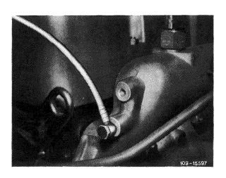
5 Unscrew fastening bracket (arrow) for oil pipe of automatic transmission.
