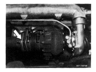
3 Unscrew engine oil feed line (1) on turbocharger and fastening clamp.
