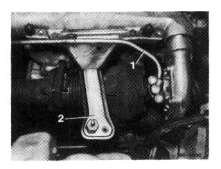
4 Unscrew pressure line to switchover valve on intake manifold.
