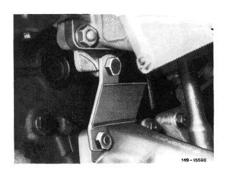
8 Unscrew fastening nuts for intake manifold and exhaust manifold, remove intake manifold and exhaust manifold together with exhaust gas turbocharger.
