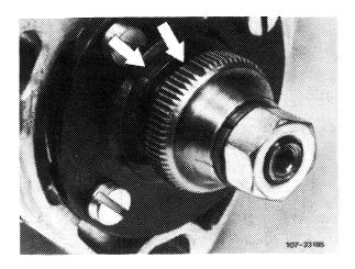
4 Slip in locking screw until there is a noticeable lock, turn camshaft slightly, if required.
