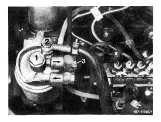
2 Release knob on hand feed pump and operate this pump until clear fuel (containing no air bubbles) emerges from union screw. Now tighten union screw again.
