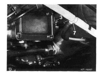
Unscrew pipe connection (1) of first injection pump element, removing compression spring (3) and delivery valve (4).
