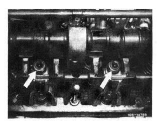
7 Set piston of 1st cylinder to TDC. Rotate crankshaft with tool combination.
