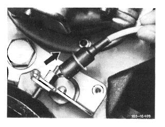
22 Place locating device without handle (arrow) into adjusting slide.
