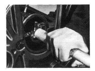
4 To obtain the required overlap, cut off radial sealing ring in cylinder crankcase and oil pan approx. 1.0 mm above parting surface.
