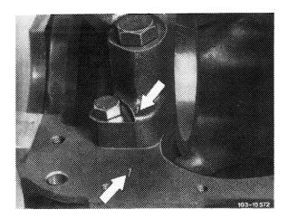
3 Measure basic bore in direction A, B and C on two levels (conicity).
