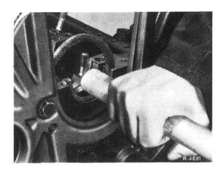
10 Provide thrust washers with engine oil and slip into grooves on fitted bearing (cylinder crankcase).
