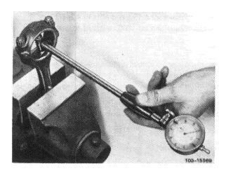
20 Insert connecting rod bearing shells, mount connecting rod bearing cap with bearing shells and tighten connecting rod nuts to 40—50 Nm.
