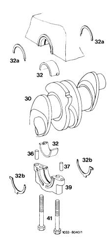
32 Bearing shells 32a Thrust washers in cylinder crankcase
