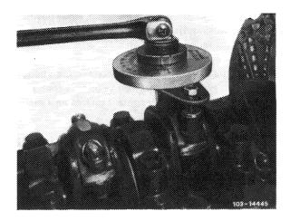
26 Measure connecting rod bearing end play. Check connecting rod for easy operation in piston.
