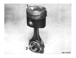
25 Tighten connecting rod nuts to 40-50 Nm initial torque and 90-100° angle of rotation torque.
