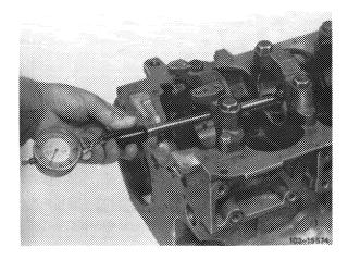
6 Measure crankshaft bearing journal, find crankshaft bearing radial play.
