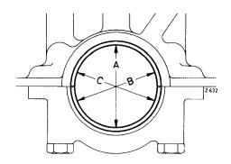
4 Insert crankshaft bearing shells and mount bearing cap. Tighten bolts to 90 Nm.
