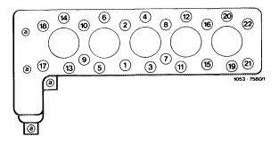
Independent of cylinder head bolt version, retightening of cylinder head bolts is no longer required during inspection 1000—1500 km or in the event of repairs after approx. 100—1500 km.
