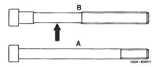
In installed condition, the cylinder head bolts are identified by the double hex. socket (B), formerly hex. socket (A).
