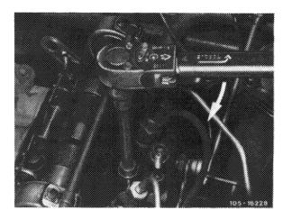
Tighten cylinder head bolts in steps in sequence of tightening diagram.
