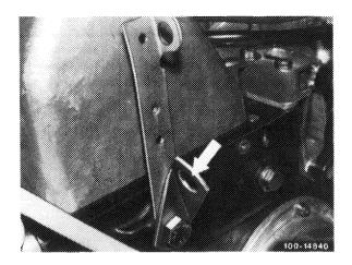
19 Lift engine as far as possible by means of engine hoist and a crane. For this purpose, on model 123, open rear clamp on air cleaner so that it will not abut against battery while lifting.
