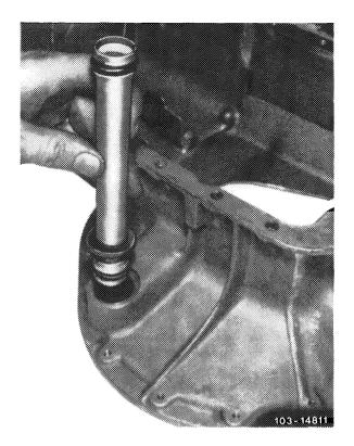
23 Renew rear radial sealing ring in oil pan according to condition.
