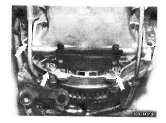
15 Knock-out oil dipstick guide tube as far as possible by means of knocking-out mandrel 9 mm dia. for valve guides.
