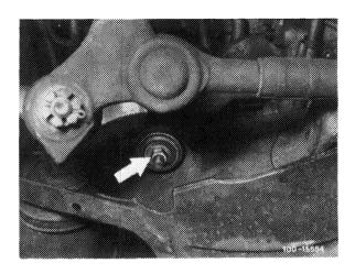
9 Loosen exhaust lateral support on transmission.
