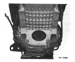
d) Oil pan upper half with integrated supporting shell and two connections for oil return line (10) from exhaust gas turbocharger and from cyclonic oil separator (8) in air cleaner.
