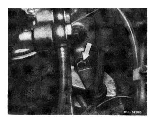
7 Slacken V-belt of refrigerant compressor and remove.
