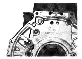
During engine repairs, the steel balls must be knocked out to clean main oil ducts.
