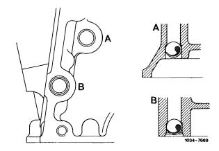
In the event of leaks, reset steel balls with knocking-in mandrel approx. 1 mm (dimension is indicated on knocking-in mandrel).
