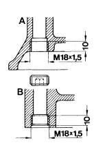
Thoroughly remove chips from oil duct.
