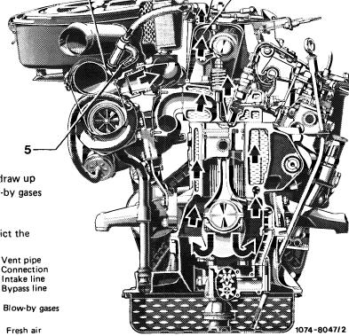
For USA Federal 1980 the vent pipe (A) screwed to inside of cylinder head cover has been replaced by a vent plate (B) which is riveted-on and sealed with silicone rubber. As a result, the volume of the oil separating space (damping chamber) has been enlarged.
