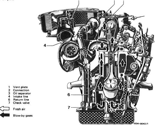
Starting model year 1981, the vent line between cylinder head cover and air cleaner has been changed from oval to round for better flow characteristics (arrow).
