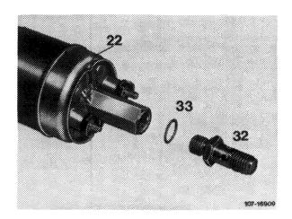
When exchanging fuel pump, make sure that the plastic sleeve is mounted in-between fuel pump and holder. Sleeve should project on both sides of holder, since direct contact of fuel pump with holder may lead to contact corrosion.
