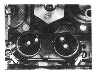
For this purpose, insert test wire of 0.5 mm dia. (arrow) into both air correction nozzles (78) one after the other and measure CO increase. CO increase should be uniformly high on both sides. Readjust with mixture adjusting screws, if required.
