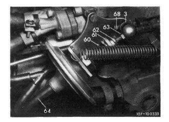
4 Check idle speed emission value without air injection. For this purpose, make air injection inoperative as follows (for 1973/74 nothing need be made inoperative):
