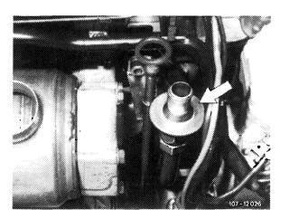
For measuring idle speed emissions, open valve plate of check valve by means of a self-made wire hook. Connect exhaust gas hose of CO measuring instrument to check valve.
