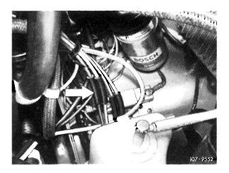
The exhaust gas for idle speed CO measurement on vehicles with catalyst, J 1976 and Ws 1975/76, is drawn off in front of catalyst at check valve (arrow) of air injection.
