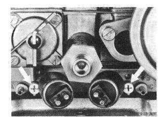
6 Check for uniform adjustment (synchronization) of mixture adjusting screws (arrows).
