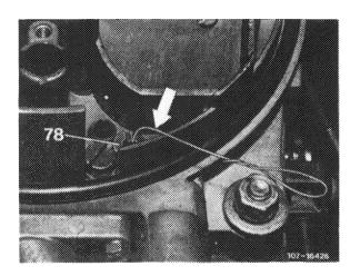
Then check whether the max. permissible idle speed emission value is not exceeded without test wire and uniformly adjust both mixture adjusting screws, if required.
