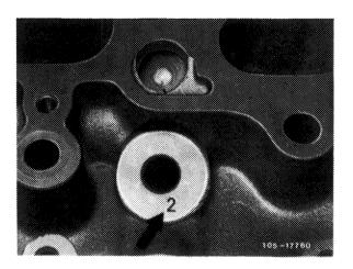
On exchange engines the basic bore in cylinder head is larger than normal. This means, that the punched-in code numbers in cylinder head are no longer in accordance with basic bores according to table.
