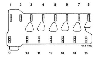
Some exchange engines are delivered with camshaft bearings in intermediate and repair sizes. This means that a standard camshaft cannot be installed in this camshaft housing, since the bearing journals are larger in diameter than the bearings.
