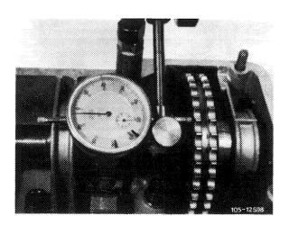
Note: If the end play is too small, grind spacing sleeve or driver at face B as required.
