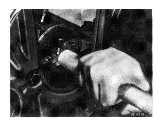
10 Provide screws on threads and on screw head contact surface with oil and tighten to 80 Nm.
