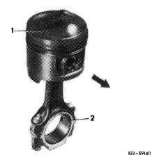
22 Tighten connecting rod nuts to 40-50 Nm initial torque and  $90-100^{\circ}$  angle of rotation.
