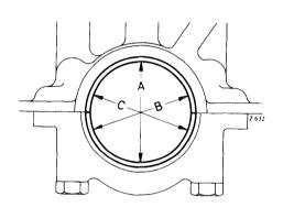
4 Insert crankshaft bearing shells and mount bearing cap. Tighten bolts to 80 Nm torque.
