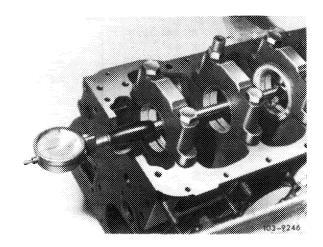
6 Measure crankshaft bearing journal, find radial crankshaft bearing play (vertical runout).
