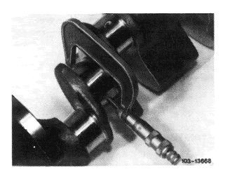
7 Measure width of fitted bearing journal and fitted bearing.
