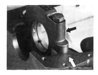
3 Measure basic bore in direction A, B and C in two levels (conicity).
