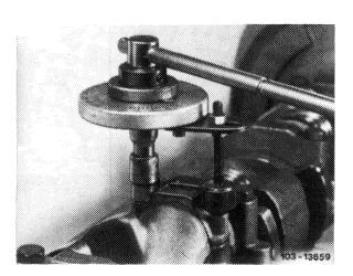
23 Measure end play of connecting rod bearing. Check connecting rod in piston for unobstructed operation.
