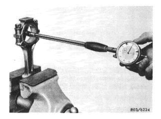
17 Insert connecting rod bearing shells, mount connecting rod bearing caps with bearing shells and tighten connecting rod nuts to 40—50 Nm.
