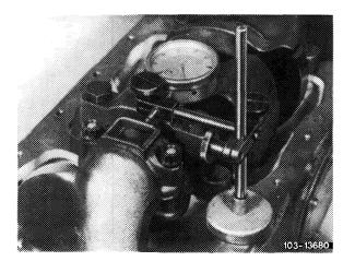
Crankshafts with riveted-on additional weight may not be used together with oil pumps, which are provided with a recess (arrow) on housing shaft.
