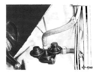
The negative vent valve opensat a slight overpressure. The evaporation vapors will flow through a line which is connected to cylinder crankcase into cylinder crankcase.
