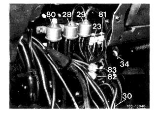
28 Switchover valve 29 Switchover valve 80 Switchover valve
