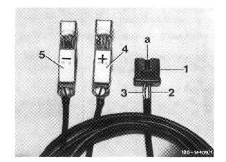
B. Temperature switch (cold engine lock)
