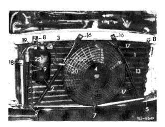
Layout of condenser with receiver dehydrator and auxiliary fan (left-hand steering)
