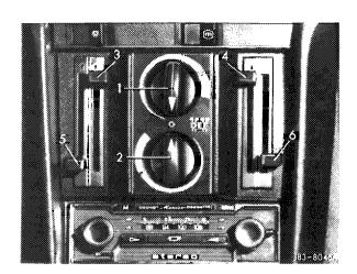
7 Check angle of rotation of temperature switch by turning knob of temperature vacuum switch (2) clockwise up to stop. The marking on knob of temperature vacuum switch should arrive at end of green key. If the angle of rotation of the temperature vacuum switch is smaller, replace temperature switch.
